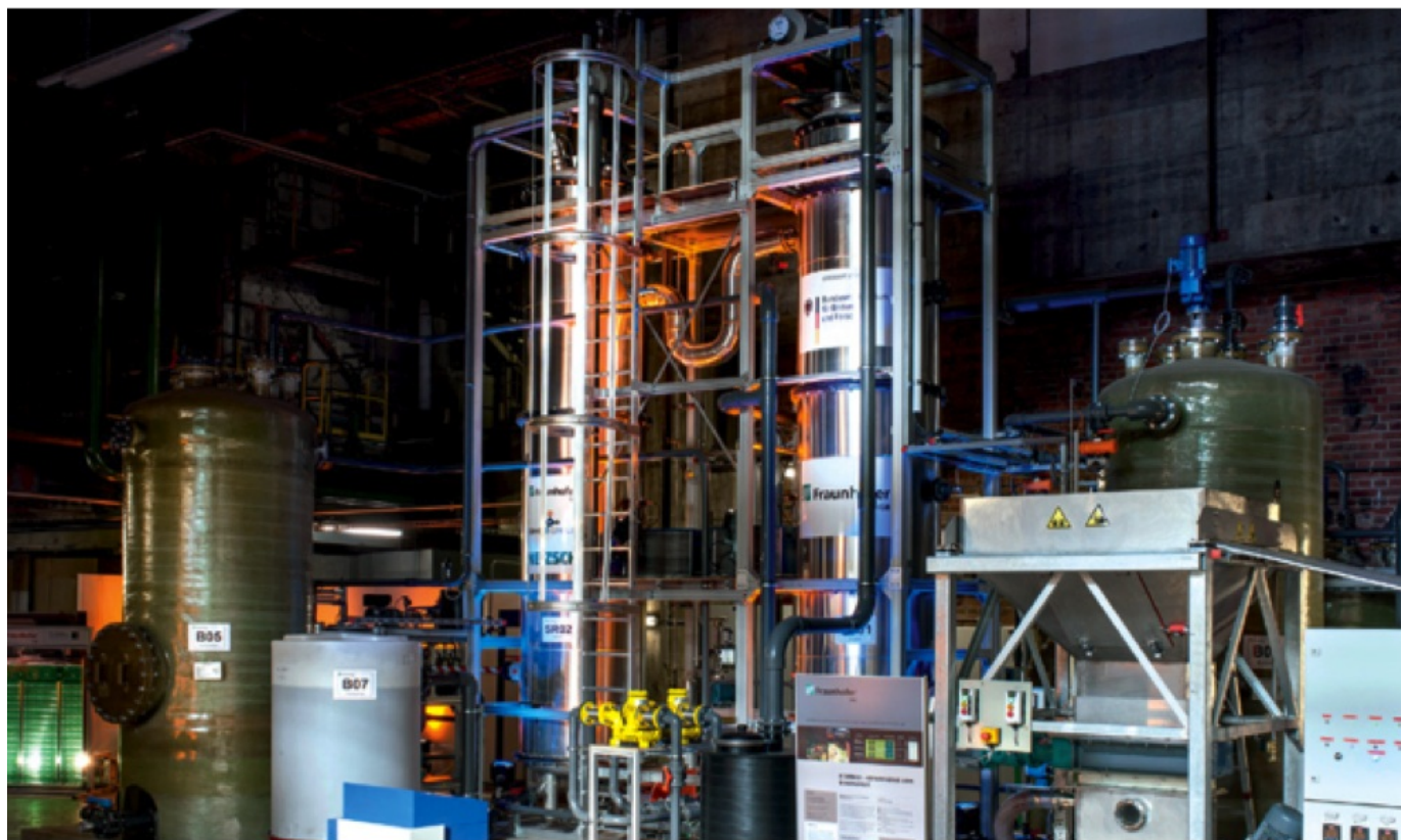
EtaMax: Production of biogas and valuable materials from fruit and vegetable waste.
