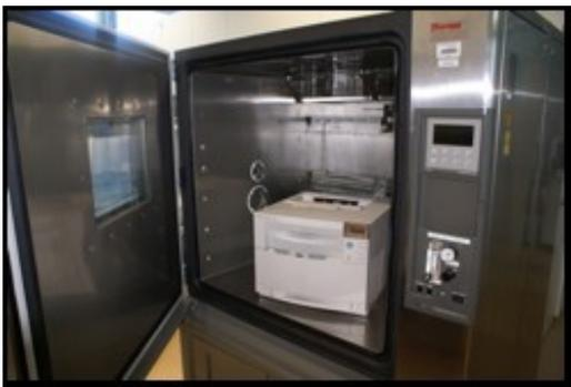
A laser printer being tested in the emission test chamber.
