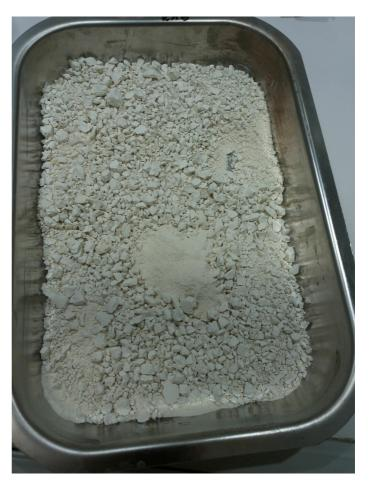
replacement material, and in a phosphate raw product, i.e. a white powder that contains phosphate. Between 80 and 100 percent of the phosphorus contained in the sewage sludge ash can be recovered using this innovative process.
