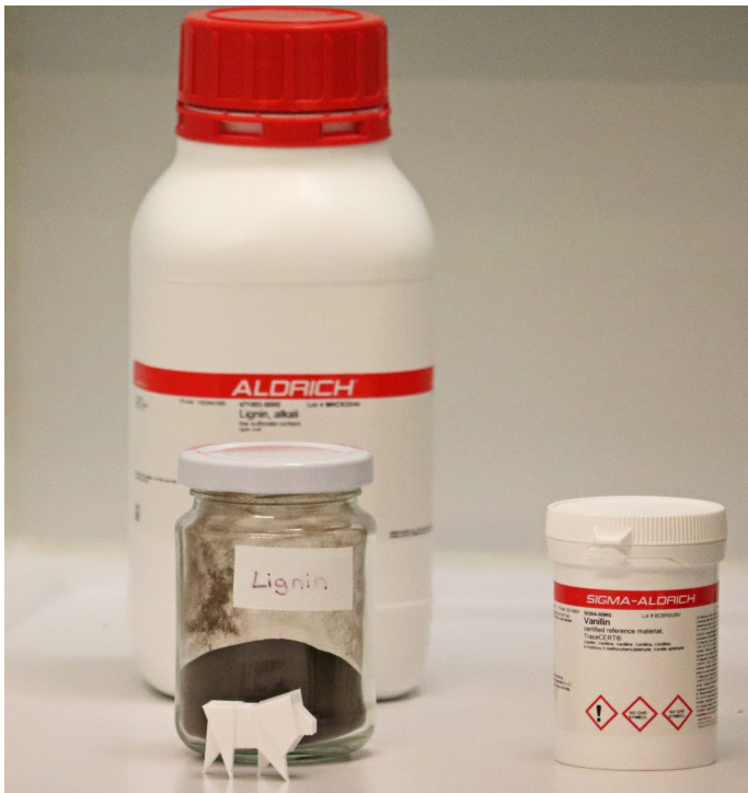
Extracting the valued flavouring substance vanillin from the biogenic residual material lignin - the InnoSÜD project is attempting to establish a new model process.
