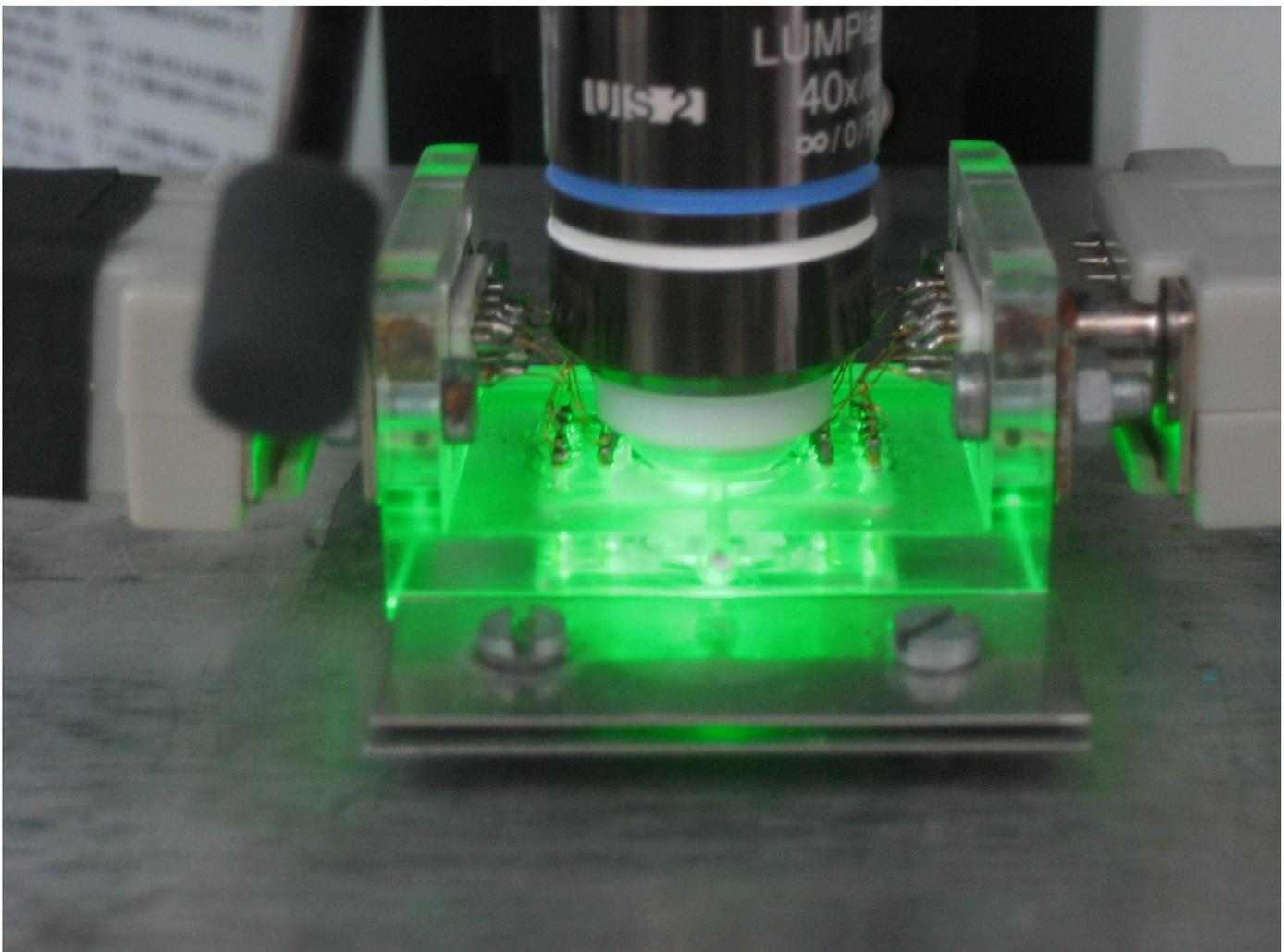
Measurements are currently carried out with a prototype. However, the serial production of nanopores on a microchip might soon become reality and be used in automated industrial processes.
