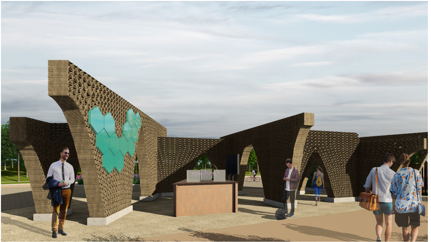
Design of the demonstration building made of willow-clay composite with integrated solar panels (green) that will be displayed at BUGA 2023 in Mannheim. © KIT-DDF
