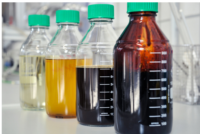
From left to right: initial solution, carbohydrate solution, HMF-rich process water and purified HMF as final product.
