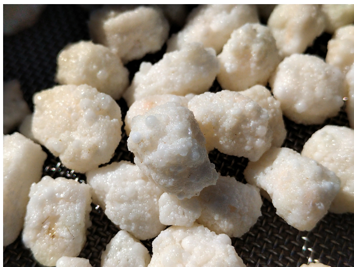
Agglomerates after successful removal process with Wasser 3.0 PE-X®. © Wasser 3.0
