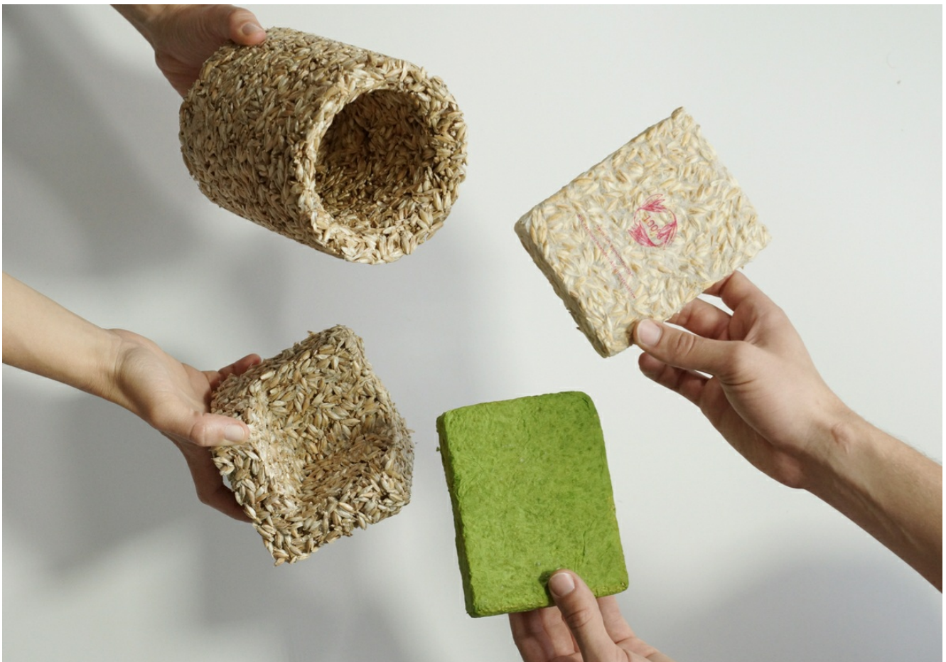
A wide variety of husks can be used for the novel packaging material and shaped into different forms depending on the application. © PROSERVATION
