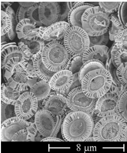
The marine algal species Emiliana huxleyi produces finely structured lime platelets that could be used for technical applications.
