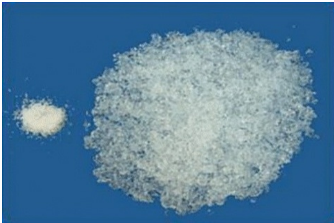
Superabsorbents made of sodium polyacrylate (left: dry; right: after absorption of water).
