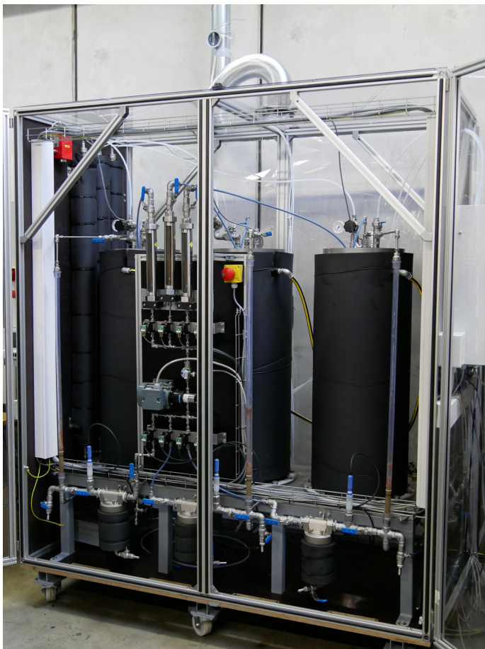
Still on a laboratory scale with 20-litre fermenters: the Hohenheim pilot facilities for the high-pressure methanation of hydrogen. Later, the real fermenters will be 100 to 500 times larger.
