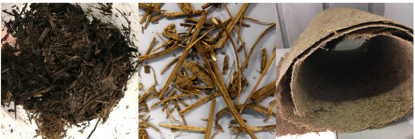
The hop fermentation residues from the biogas plant are washed and then processed into a fleece. © DITF
