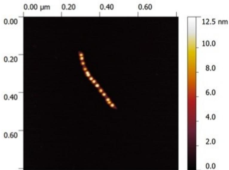
DNA nanotube 400 nm long, conjugated with 10nm-long silver nanoparticles. It can be used for guiding light rays in specific directions.
