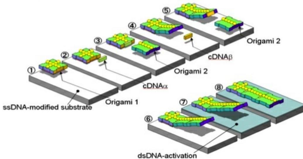
The DNA origami method enables the researchers to fold DNA molecules into complicated scaffolds.
