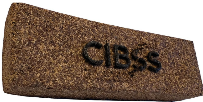
Bacteria can be used to create sustainable biocomposites with a wide variety of properties from wood waste.
