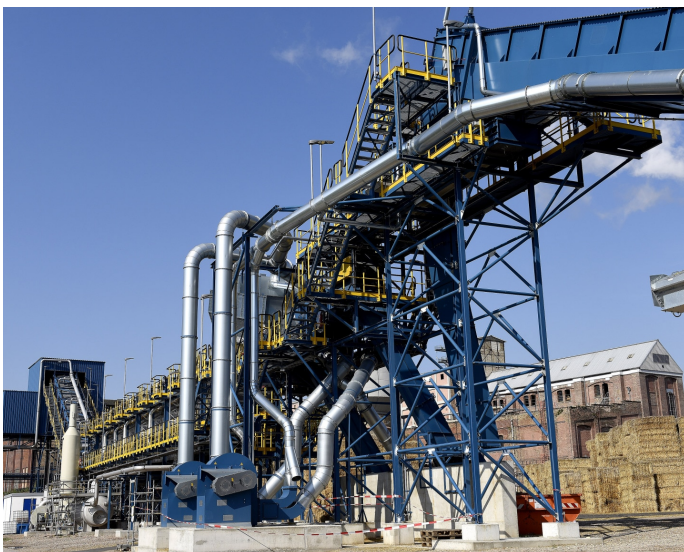
A huge straw conveyor belt takes the bales directly from the storage yard to production. © Essity/Tröster
