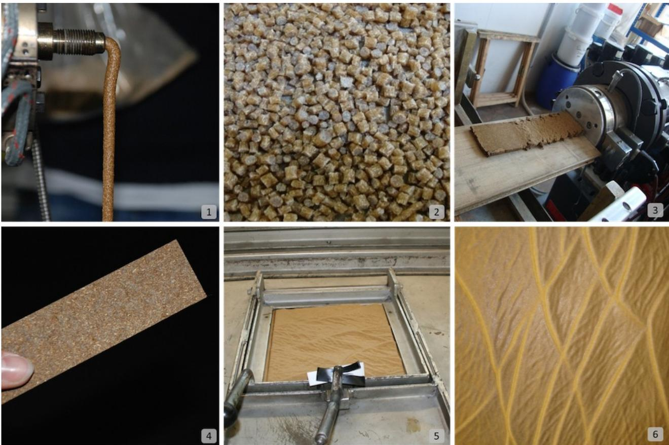
Production of a natural fibre-based material: compounding (mixing of plastic with natural fibres, pelletising) (1) (2), extrusion of the tough mass through a mould (3) (4) and thermal deep-drawing of the material to achieve the sought-after design (5) (6)
