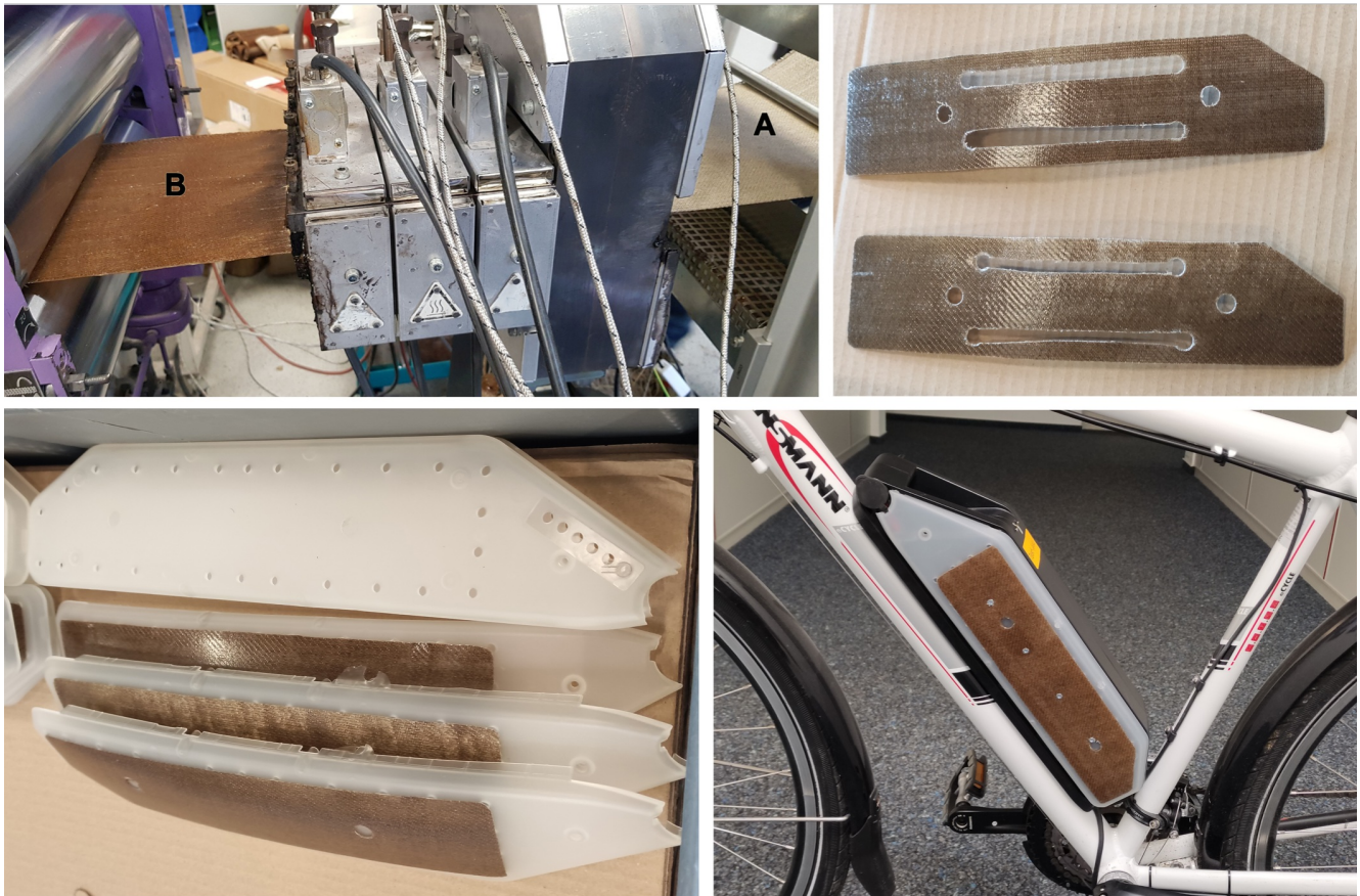
Thin organo sheets (B) are made from flax fabric (A) and polypropylene, which are used to reinforce the panels of an e-bike battery case. © Ansmann AG & Fraunhofer LBF
