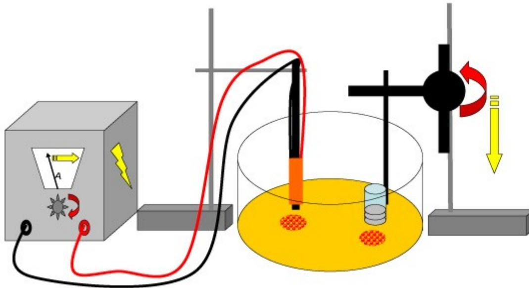
Magnetic particle induction, MagPI for short, can be used to analyse the adhesive power of biofilms. Dr. Sabine Ulrike Gerbersdorf is very keen on the idea of developing the principle into a new device. The schematic shows two application variants. In the variant on the right, the distance of the magnet to the surface can be varied, and in the variant on the left, the supply of electricity can be varied.
