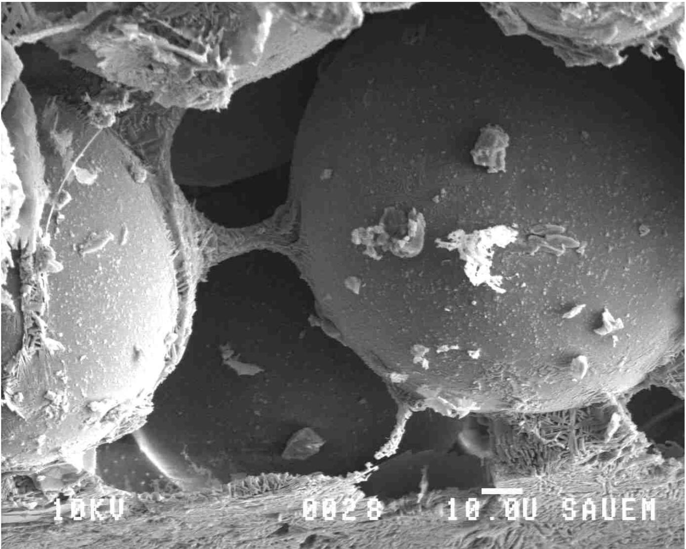
Electron microscope image shows in detail how the bacterial biofilm links glass spheres with each other
