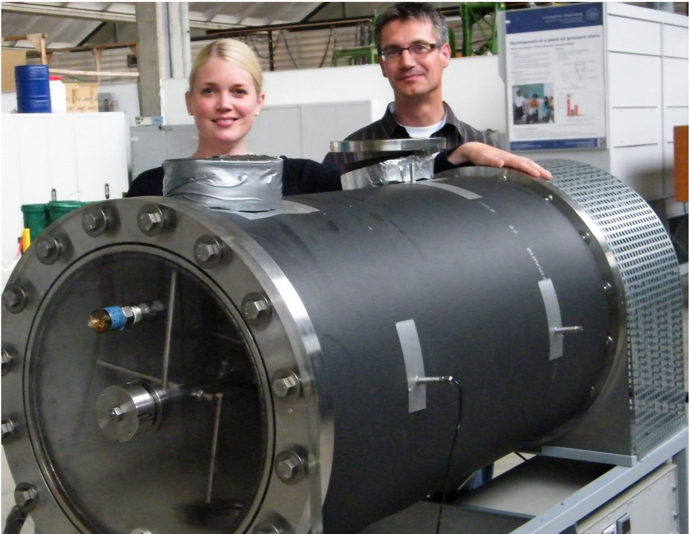
Doctoral student Friederike Hahn and Dr. Andreas Lemmer are testing new methods for the production of biogas. The two researchers are standing behind a fermenter prototype that is being used for primary fermentation.
