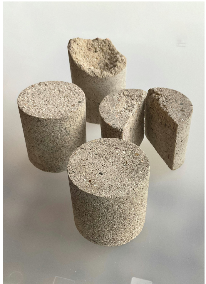
The bioconcrete test specimens produced by microbiologically induced calcite precipitation already have a high compressive strength. © ILEK, University of Stuttgart
