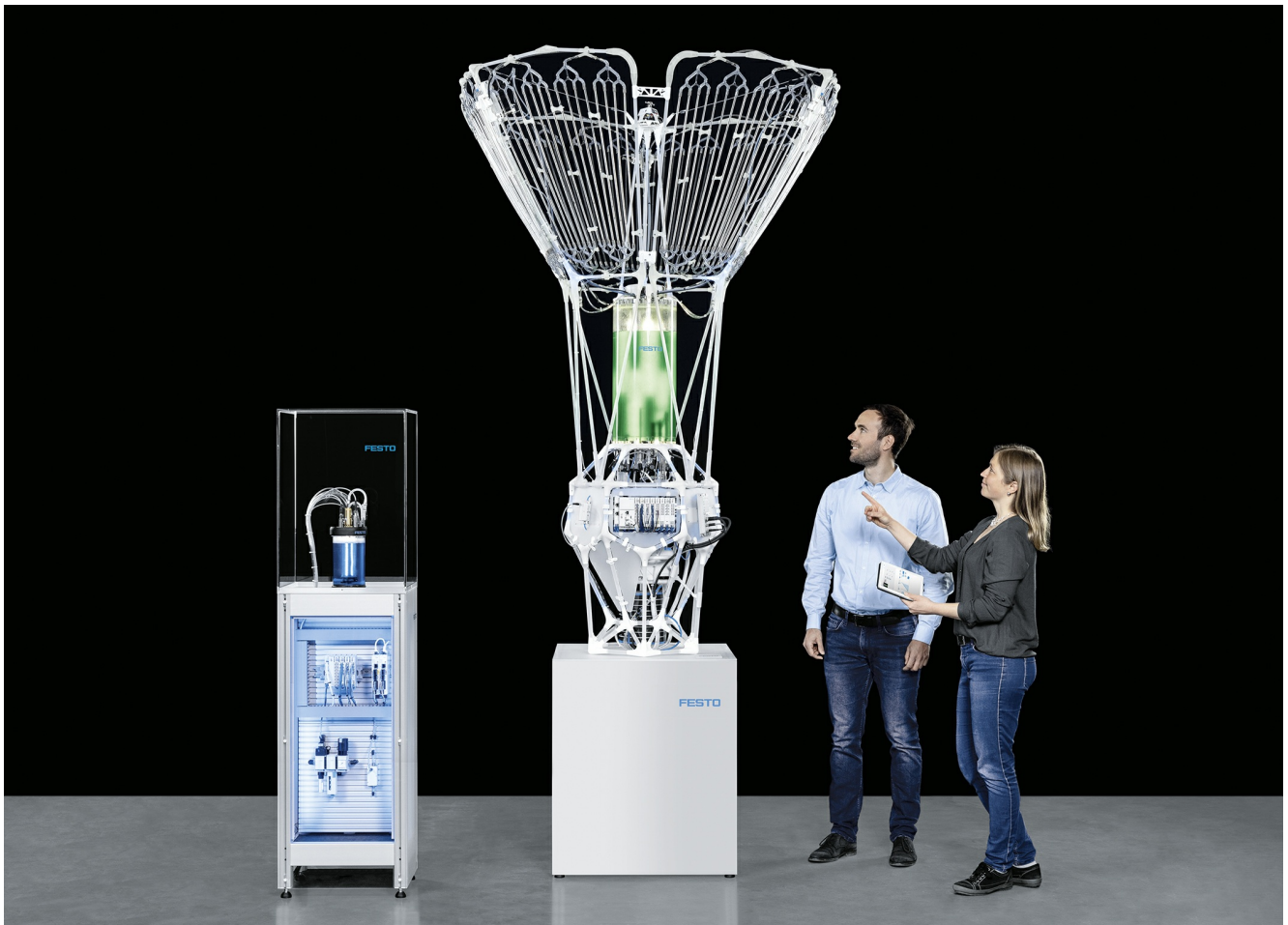
Festo has developed the PhotoBionicCell bioreactor in which biomass can be cultivated automatically. © Festo SE & Co. KG
