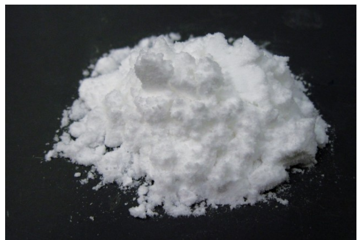
Struvite extracted from wastewater and used as a slow-release nitrogen and phosphorus fertiliser. © Fraunhofer IGB
