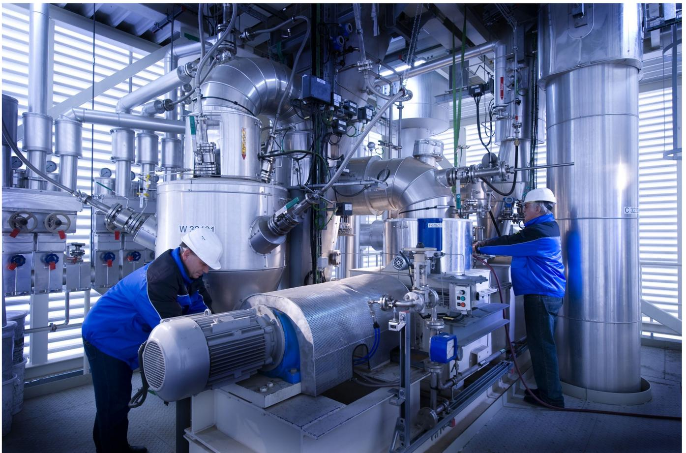
Reactor for the production of bioliqSynCrude<sup>®</sup> on the northern KIT campus – the first stage of the bioliq<sup>®</sup> process
